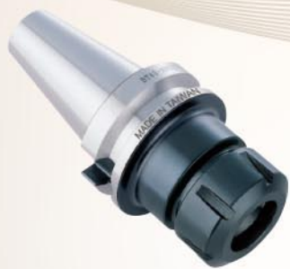
BT Shank JIS B 6339(MAS 403 BT) with Collet Chuck DIN 6499
