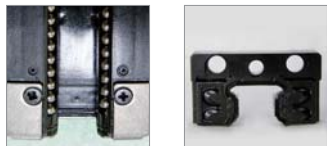
Plastic parts in good condition End seal in good condition
